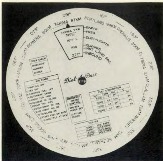
Left, one side has major emergency procedures and a window to read facilities information pertinent to base dialed. Right, reverse is devoted to unit navigation. Below, mileage chart gives distances, vectors to bases.
