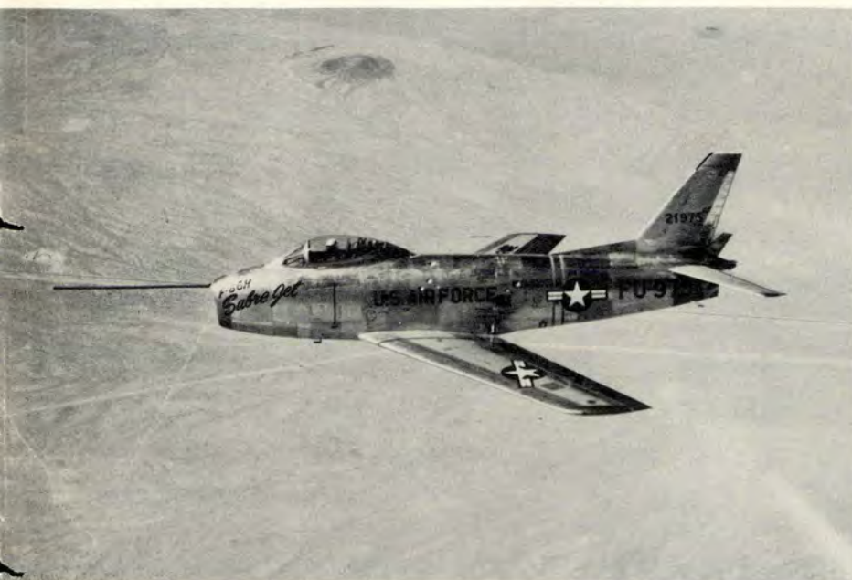
Below is the fifth and latest of the F-86's—the H. The cannon-like object protruding from F-86H nose is an airspeed boom used only in flight test work to make exact airspeed calibrations.
